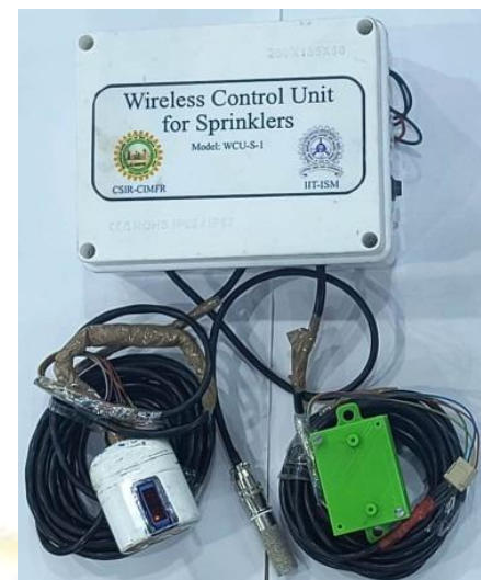
Fig.3: Control unit with sensors for sprinklers operation
