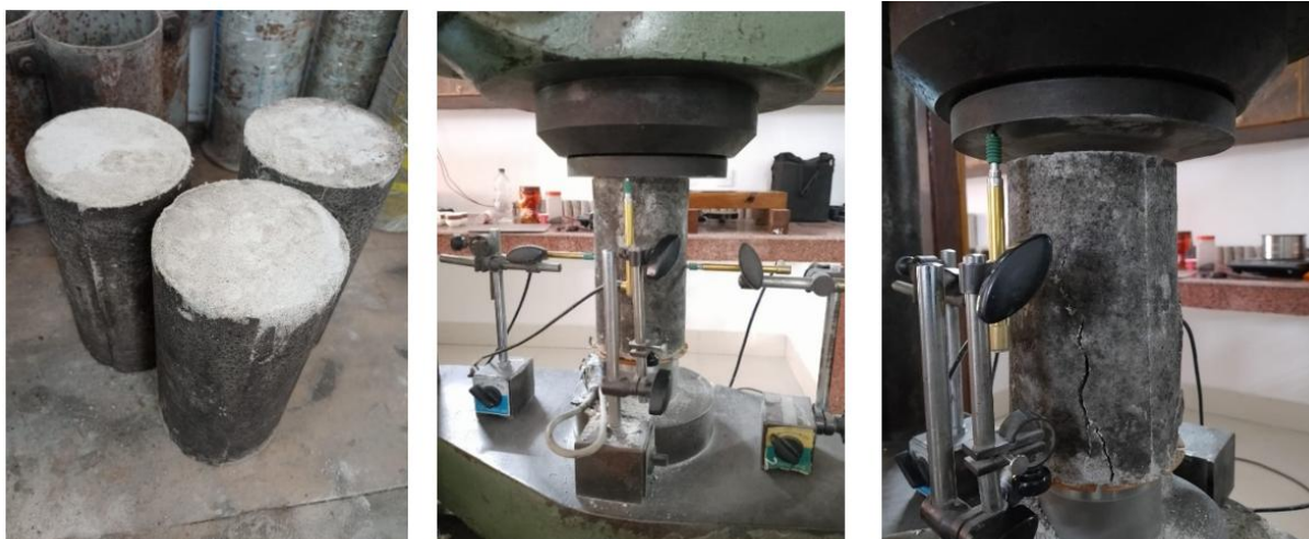
Sample preparation and determination of USC, YM, PR
