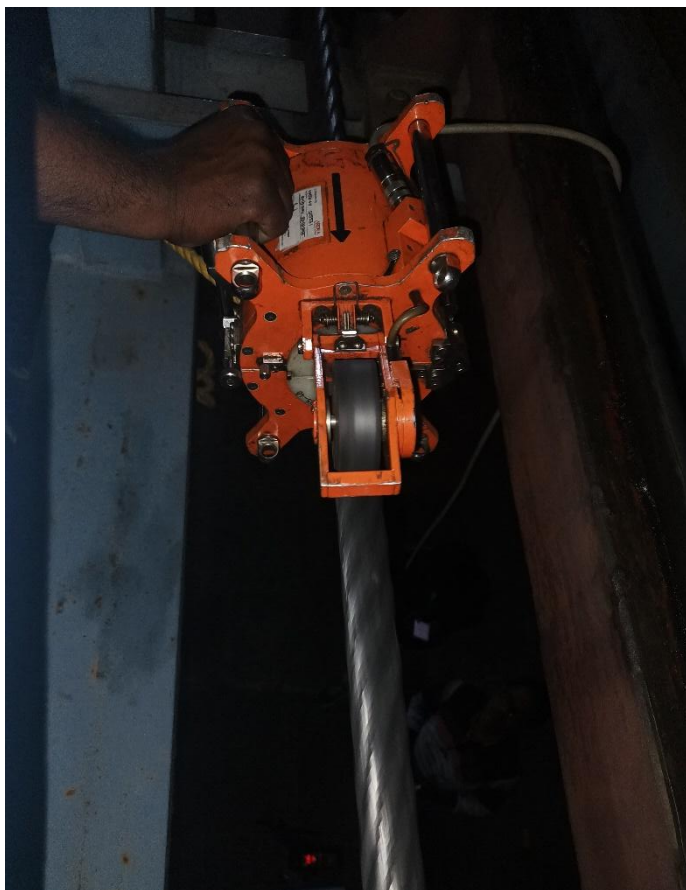
Wire rope testing instrument mounted on a moving steel wire rope for condition monitoring.
