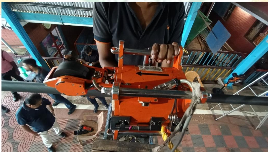
Scanning of Steel Wire Rope in progress at Malampuzha Ropeway, Pallakad, Kerala
