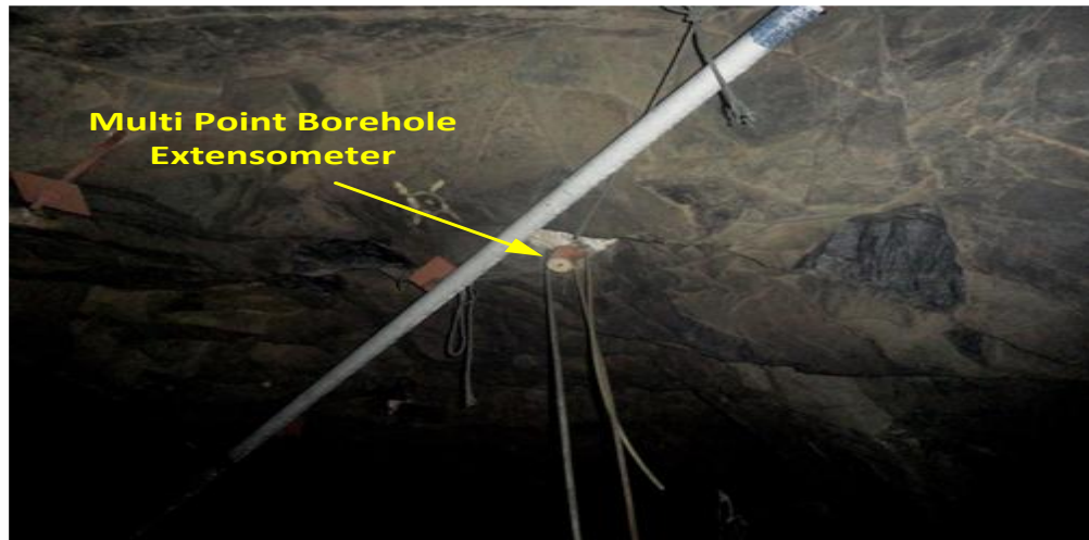
Fig. 6: Multipoint Borehole Extensometer installed in the crown pillar of the already extracted 12-15 stope at 174mRL.
