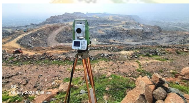
Geo-reference establishment by Total Station
