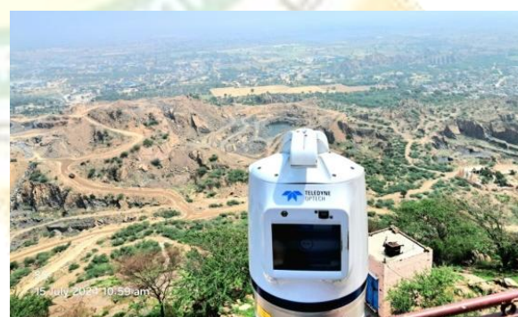
Survey by Terrestrial Laser Scanner
