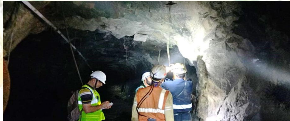
Fig. 7: Reading taken from Vibrating wire type stress meter installed in the crown Pillar of already extracted stopes P-V-B-12-14A/12-15 at 174mRL.
