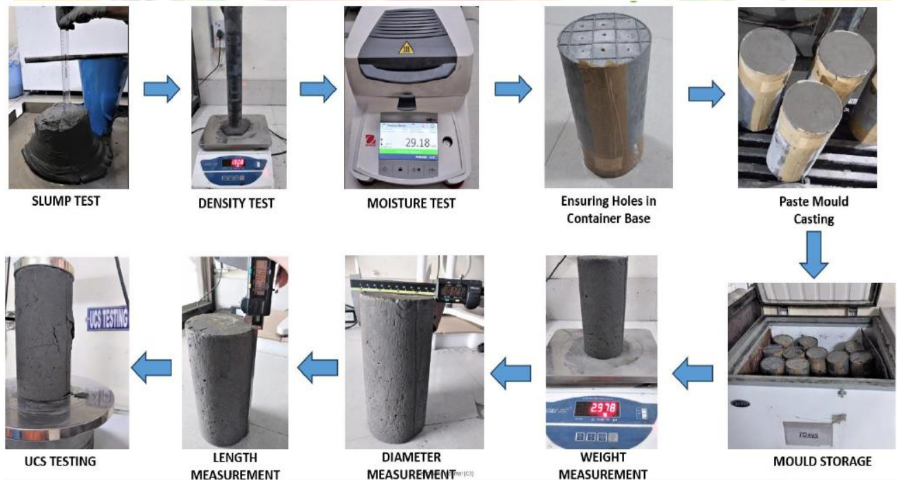
Fig. 11: Procedure followed in laboratory for determining the strength of paste fill material.
