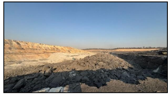
Fig.3: View of casting of rock from dozer-push operation
