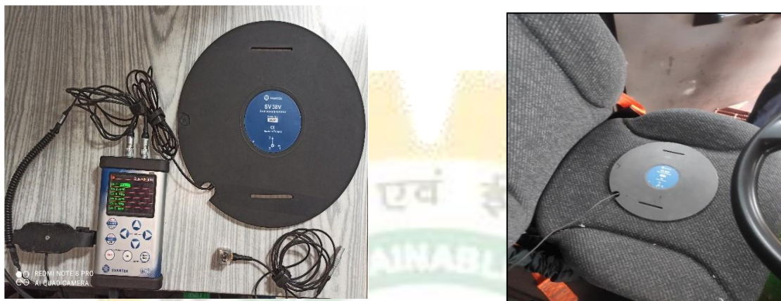
Fig.5: Whole body vibration meter and seat pad accelerometer.
